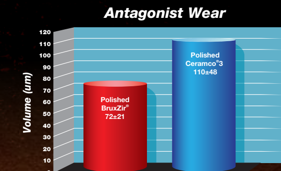
The antagonistic (Steatite balls) wear shows BruxZir only with 72±21 micron, which is significantly lower than Ceramco® 3 (110±48 micron). The University of Tübingen study was run using an eight chamber Willytec Chewing Simulator at 1.2 million cycles.
